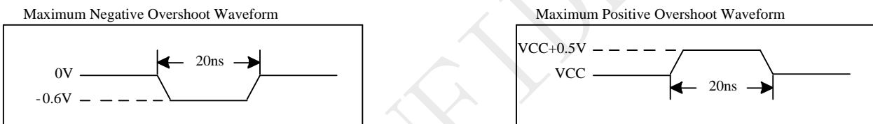
Figure 5-1 Maximum Overshoot Waveform
