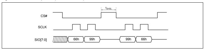
Figure 116. Reset Sequence (DTR-OPI mode)
