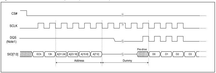
Note1: DQS is enabled only when DOS (DQS on STR mode) bit is set. Otherwise, it keeps Hi-Z.
