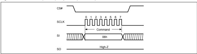
Figure 6. Write Enable (WREN) Sequence (STR-OPI Mode)
