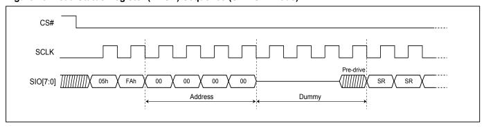
Figure 16. Read Status Register (RDSR) Sequence (DTR-OPI Mode)
