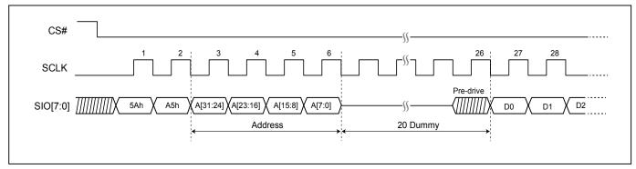
Figure 119. Read Serial Flash Discoverable Parameter (RDSFDP) Sequence (DTR-OPI Mode)
