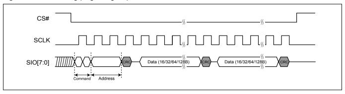
Figure 124. CRC Timing (Write Register - example for 1byte data)
