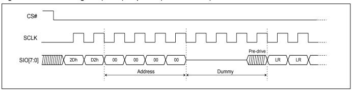
Figure 82. Read Lock Register (RDLR) Sequence (DTR-OPI Mode)
