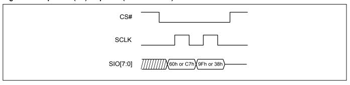
Figure 69. Chip Erase (CE) Sequence (DTR-OPI Mode)
