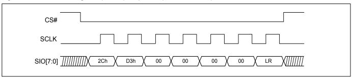
Figure 85. Write Lock Register (WRLR) Sequence (DTR-OPI Mode)
