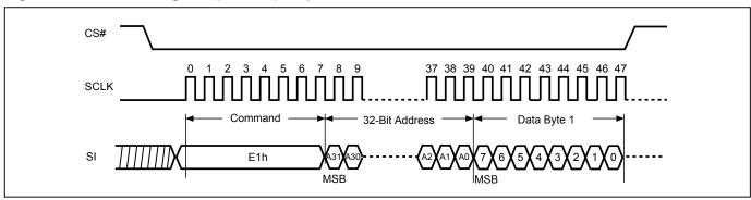
Figure 98. Write DPB Register (WRDPB) Sequence (STR-OPI Mode)
