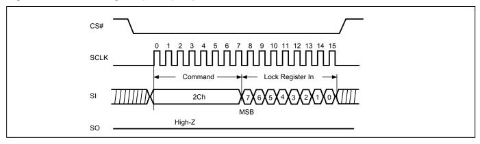
Figure 84. Write Lock Register (WRLR) Sequence (STR-OPI Mode)
