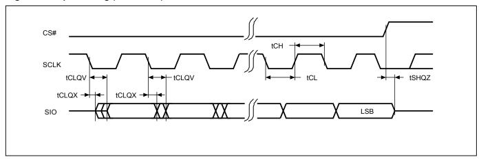
Figure 4. Output Timing (DTR mode)
