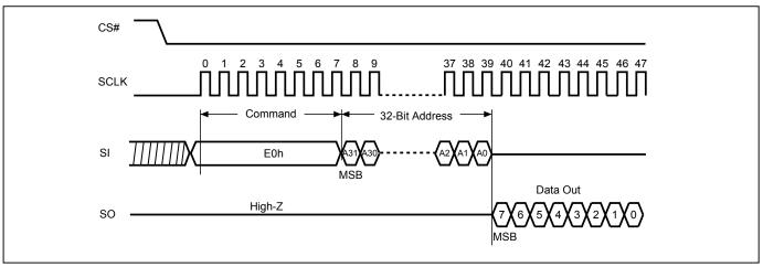
Figure 96. Read DPB Register (RDDPB) Sequence (STR-OPI Mode)
