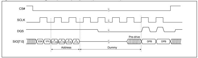
Figure 97. Write DPB Register (WRDPB) Sequence
