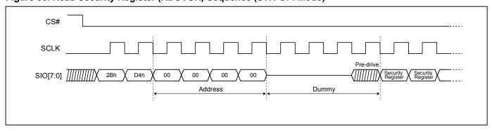
Figure 36. Read Security Register (RDSCUR) Sequence (DTR-OPI Mode)
