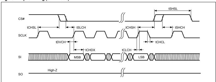
Figure 2. Input Timing (DTR mode)
