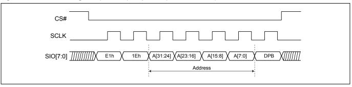
Figure 100. Write DPB Register (WRDPB) Sequence (DTR-OPI Mode)
