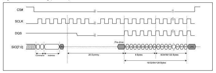
Figure 127. CRC Timing (WRPASS/PASSULK)
