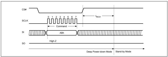
Figure 77. Release from Deep Power-down (RDP) Sequence (STR-OPI Mode)
