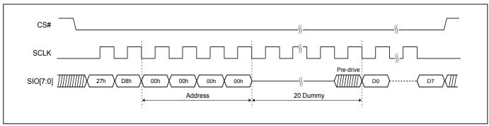
Figure 103. Read Password Register (RDPASS) Sequence (DTR-OPI Mode)
