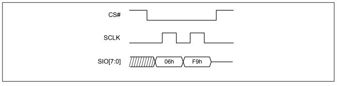
Figure 7. Write Enable (WREN) Sequence (DTR-OPI Mode)
