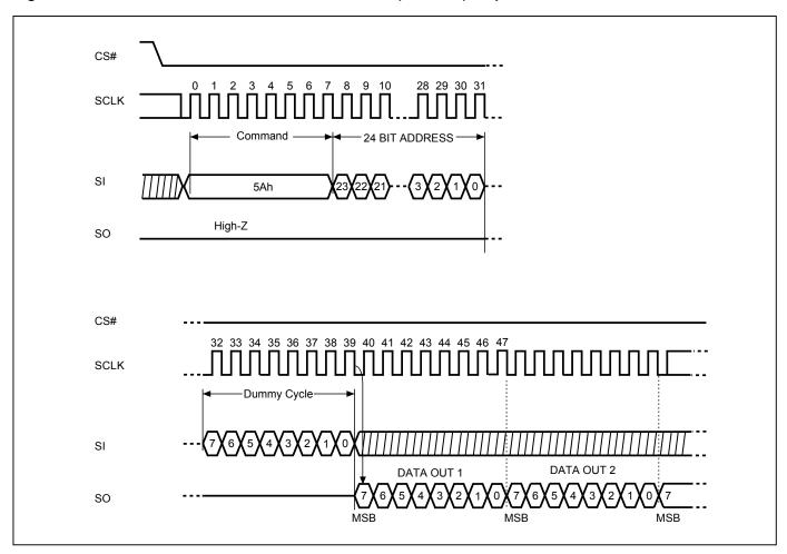
Figure 118. Read Serial Flash Discoverable Parameter (RDSFDP) Sequence (STR-OPI Mode)
