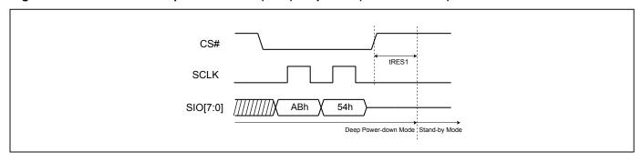
Figure 78. Release from Deep Power-down (RDP) Sequence (DTR-OPI Mode)
