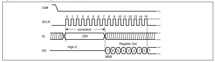
Figure 81. Read Lock Register (RDLR) Sequence (STR-OPI Mode)
