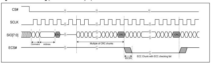
Figure 122. CRC Timing (With CRC# output)
