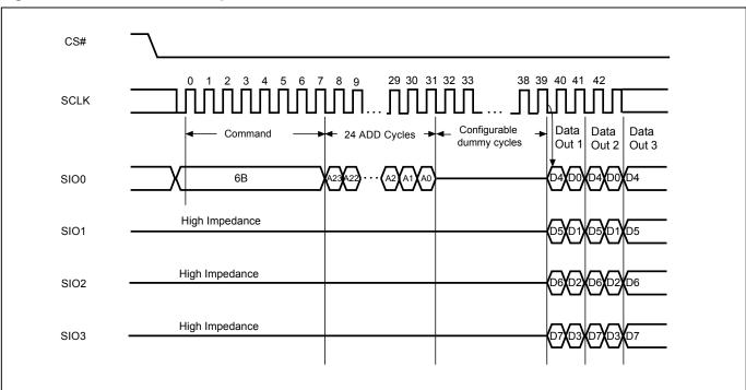
Figure 31. Quad Read Mode Sequence
