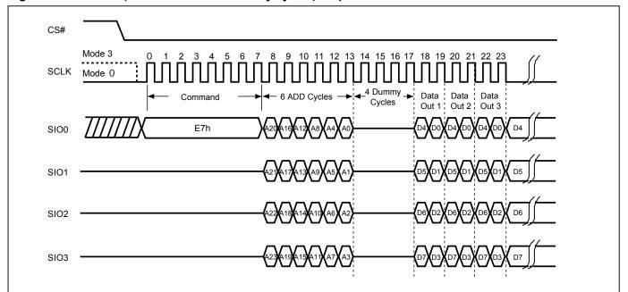
Figure 32. W4READ (Quad Read with 4 dummy cycles) Sequence
