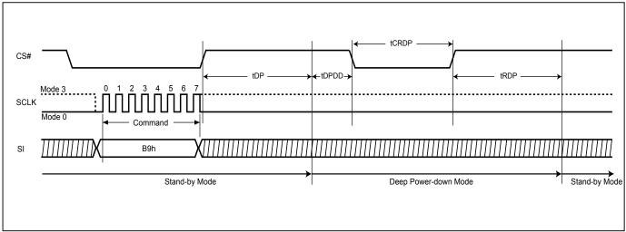
Figure 55. Deep Power-down (DP) Sequence and Release from Deep Power-down Sequence (QPI Mode)
