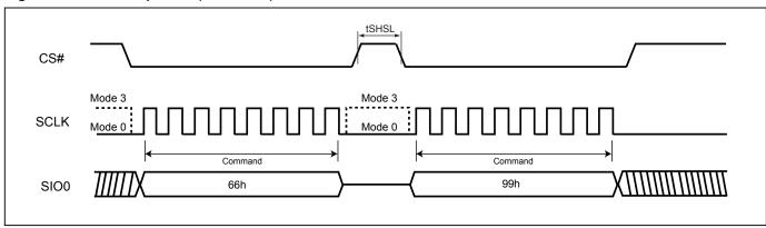
Figure 76. Reset Sequence (QPI mode)
