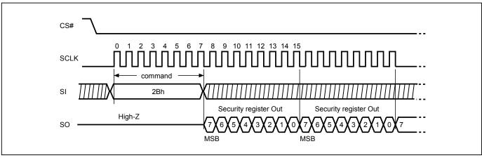
Figure 57. Read Security Register (RDSCUR) Sequence (QPI Mode)
