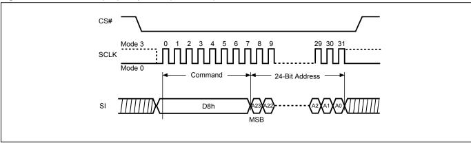
Figure 44. Block Erase (BE) Sequence (QPI Mode)
