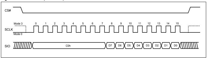
Figure 36. Burst Read (QPI Mode)
