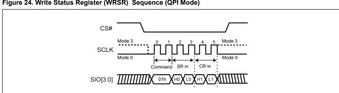
Figure 24. Write Status Register (WRSR) Sequence (QPI Mode)
