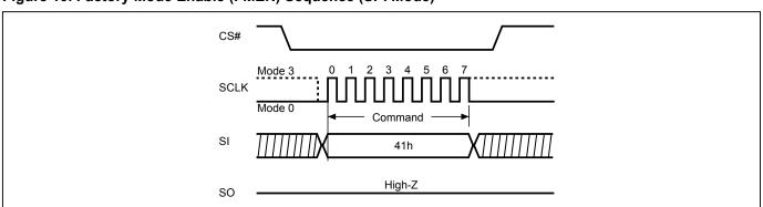
Figure 12. Factory Mode Enable (FMEN) Sequence (QPI Mode)
