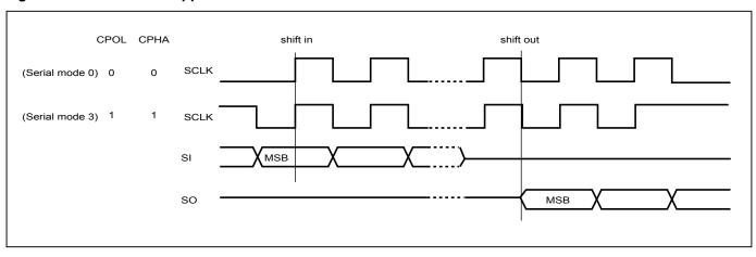
Figure 1. Serial Modes Supported
