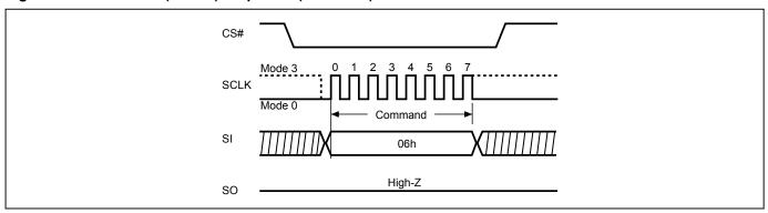
Figure 7. Write Enable (WREN) Sequence (QPI Mode)
