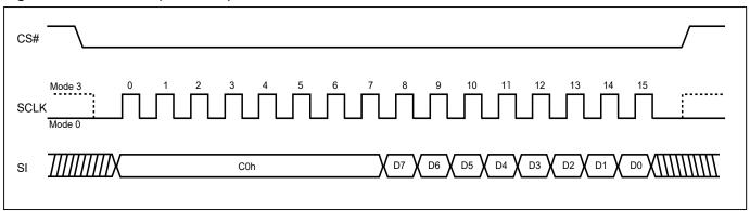
Figure 35. Burst Read (QPI Mode)
