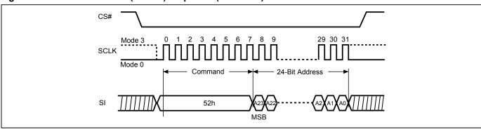
Figure 41. Block Erase 32KB (BE32K) Sequence (QPI Mode)
