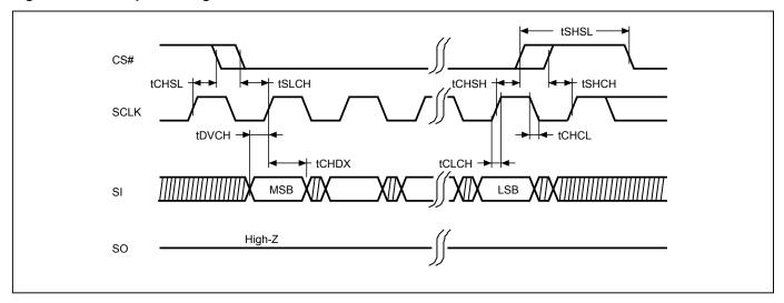
Figure 3. Output Timing
