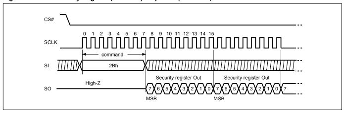
Figure 56. Read Security Register (RDSCUR) Sequence (QPI Mode)
