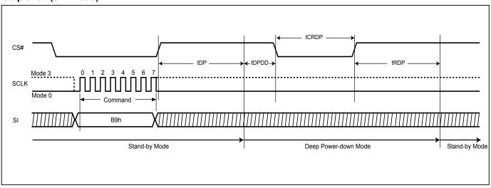
Figure 54. Deep Power-down (DP) Sequence and Release from Deep Power-down to enter Standby Mode Sequence (QPI Mode)
