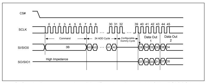
Figure 28. Dual Read Mode Sequence (SPI Mode only)
