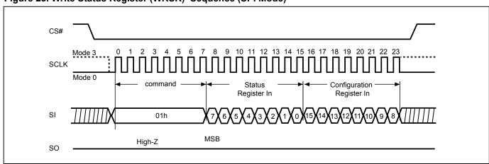
Figure 23. Write Status Register (WRSR) Sequence (SPI Mode)
