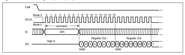
Figure 63. Write Lock Register (WRLR) Sequence
