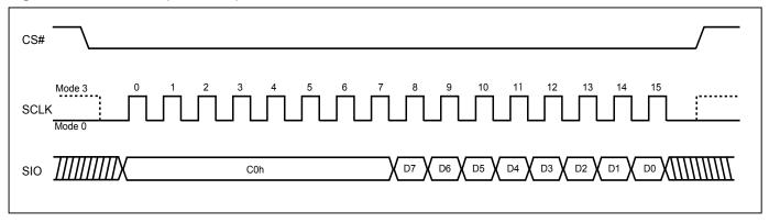
Figure 62. Burst Read (QPI Mode)
