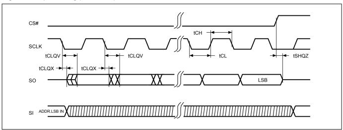
Figure 4. Output Timing (DTR mode)
