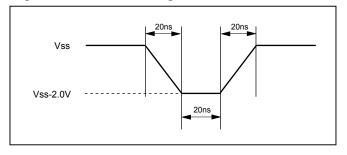
Figure 103. Maximum Positive Overshoot Waveform
