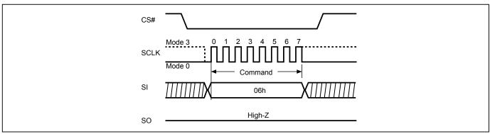
Figure 13. Write Enable (WREN) Sequence (QPI Mode)
