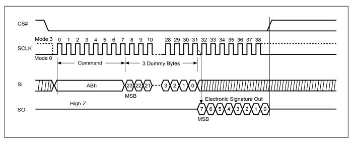
Figure 18. Read Electronic Signature (RES) Sequence (QPI Mode)
