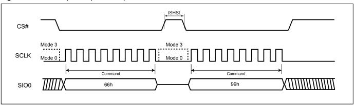
Figure 99. Reset Sequence (QPI mode)
