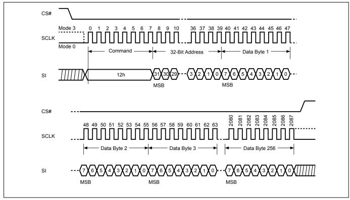
Figure 56. 4 x I/O Page Program (4PP4B) Sequence (SPI Mode only)
