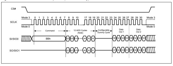
Figure 33. 2 x I/O Read Mode Sequence (SPI Mode only)
