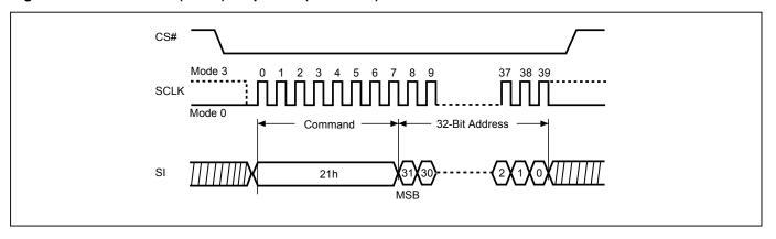
Figure 53. Block Erase 32KB (BE32K4B) Sequence (SPI Mode)
