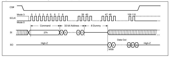
Figure 91. Write Password Register (WRPASS) Sequence
