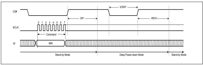
Figure 80. Deep Power-down (DP) Sequence (QPI Mode)
