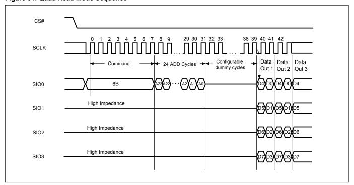
Figure 34. Quad Read Mode Sequence
