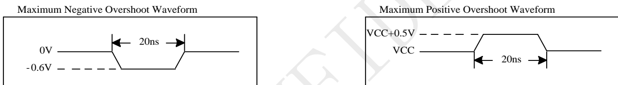
Figure 5-1 Maximum Overshoot Waveform
