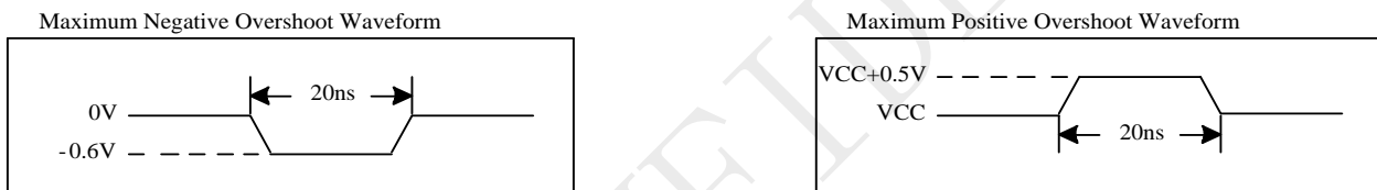
Figure 5-1 Maximum Overshoot Waveform
