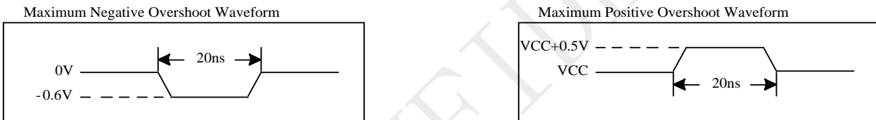
Figure 5-1 Maximum Overshoot Waveform
