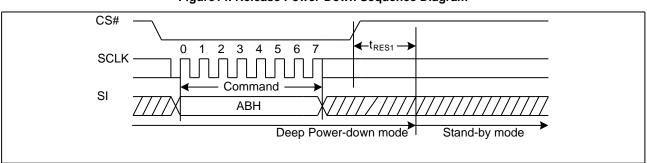
Figure 14. Release Power-Down Sequence Diagram
