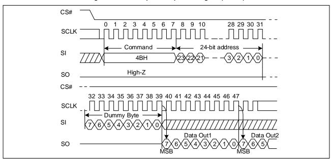
Figure 18. Read Unique ID Sequence Diagram (ADS=0)
