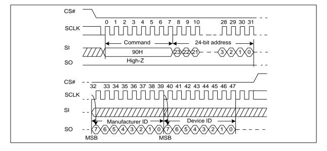
Figure 16. Read Manufacture ID/ Device ID Sequence Diagram
