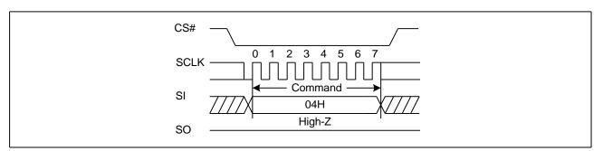
Figure 2. Write Disable Sequence Diagram
