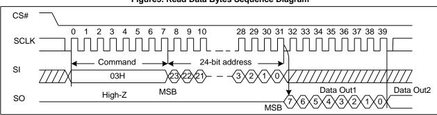
Figure 5. Read Data Bytes Sequence Diagram
